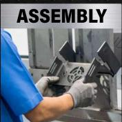
Assembly involves combining fabricated metal components, sometimes with non-metal elements like fasteners or gaskets, to create a finished product.
